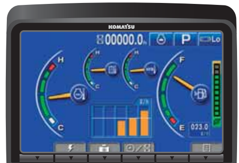
Eco-gauge, idle caution and adjustable idle shut-down to further reduce fuel consumption
