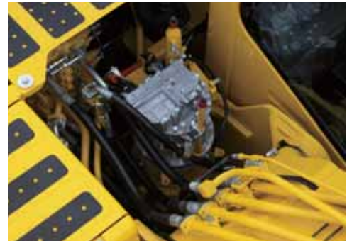
An electric swing motor is used in place of the usual hydraulic swing motor and is designed to recover energy during swing braking.
