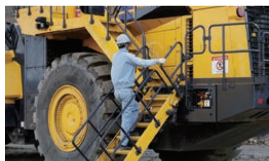
Power ladder (optional) provides safer access and egress.
